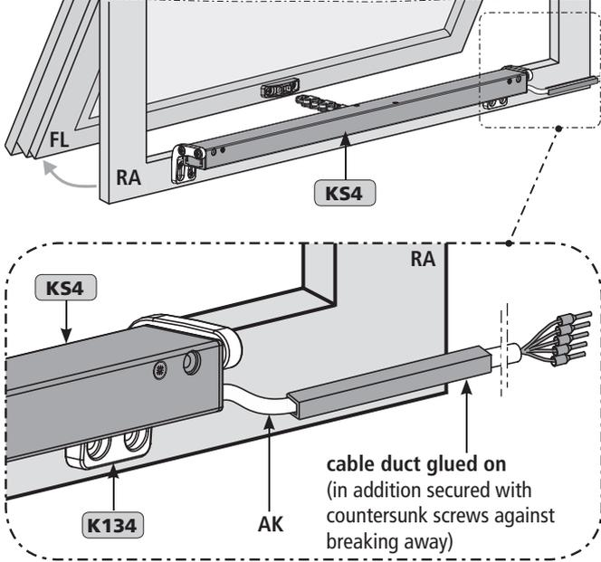
cable duct glued on (in addition secured with countersunk screws against breaking away)
