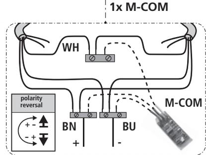
A maximum of three individual drives and one locking drive in series connection possible. Configuration is done by M-COM.
