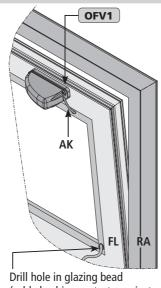
(cable bushing protects against damage to cable).
