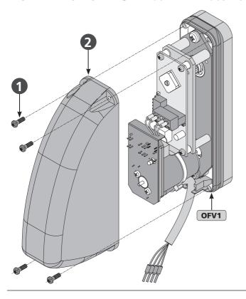
■ Using the screws **①** and mount the housing **②** on the locking drive **OFV1**.
