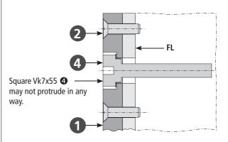
■ Insert the locking drive **OFV1** into groove of square Vk7x55 **4** and fasten it with two screws **5** and spring rings **6** on the adapter plate **1**.
