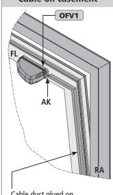
Cable duct glued on (in addition secured with countersunk screws against breaking away).
