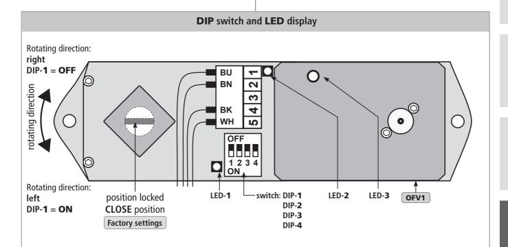
**Note** In case of wrong direction of rotation, reverse polarity from the <u>opening drive</u>.
